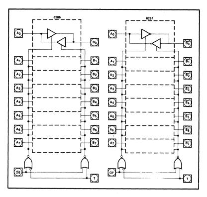
Figure 3. Logic Diagrams
